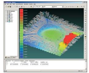
Ansoft offers SIwave™ v2, a full-wave EM tool for detailed signal and power integrity analysis.
